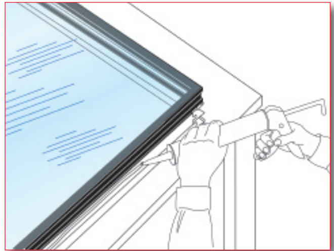
Fig. 17: Weather sealant application
